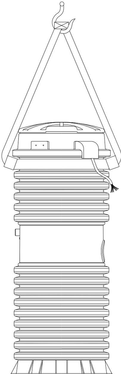
2. No Ballast (to be poured in place): If the concrete anchor is to be poured while the station is in place lift the unit using 2 nylon straps wrapped around the accessway making a sling, as shown below. Keep station oriented vertically to avoid any damage. Only lift from the accessway to put unit in hole, not for moving any distance.
